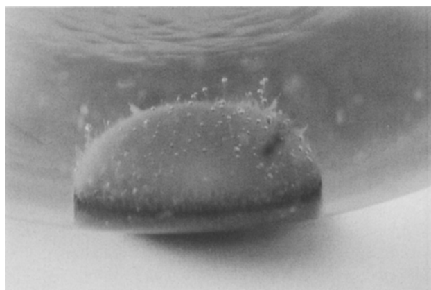
Figure 2. Visual observation of S. lipolytica biofilm on Mexphalte R 90/40.
